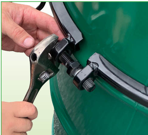
5 Keeping THE JACK in position, tighten the main bolt.
