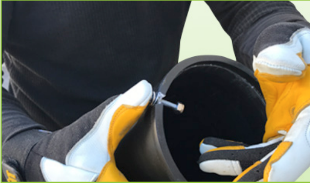
1 Loosen and remove bolt and nut from the S'HUSH Silencer and store in a safe place.
