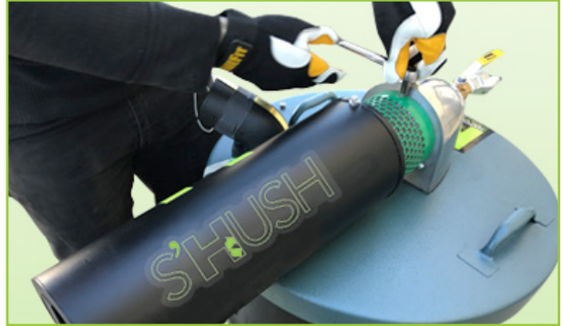
2 Loosen Anchor Screw and remove from Venturi head with 3/8" wrench. Slide S'HUSH onto the head.
