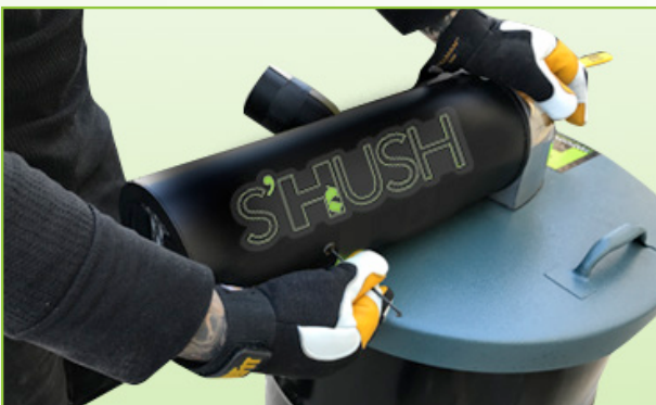
5 Insert bolt on right and loosely tighten with included allen wrench.
